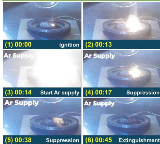
Experiment of lithium ignition and extinguishing. The ignition temperature was around 600 degree under
