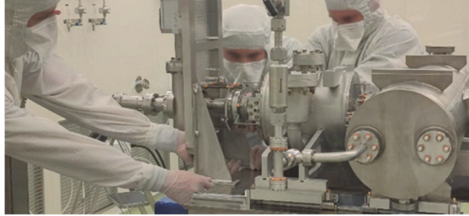
FIG. 9. Installation of the component of the beam line in the clean room.
