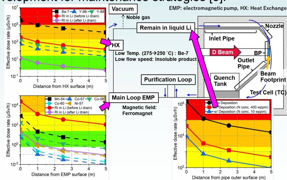
Effective doses around the Li-loop components due to the radionuclide in the liquid Li and deposits. [4] Kenjo S et al., Fus. Eng. Des. (2024)
