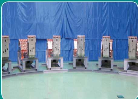
Divertor cassette bodies at the Naka Fusion Institute before mounting with plasma-facing components.
