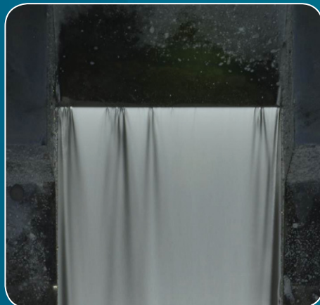
Flowing lithium in the ELTL facility (Oarai)
